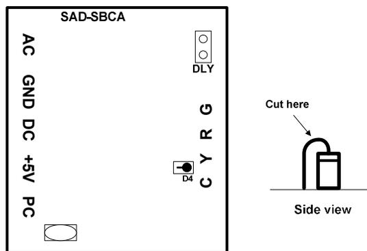
Figure 5 – cutting diode D4 for absolute type signals
