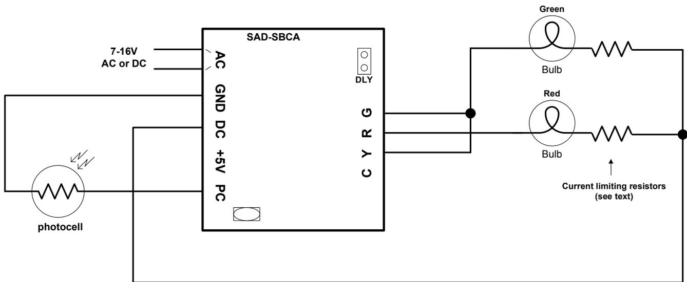
Figure 3 – 2-light bulb-based signals
