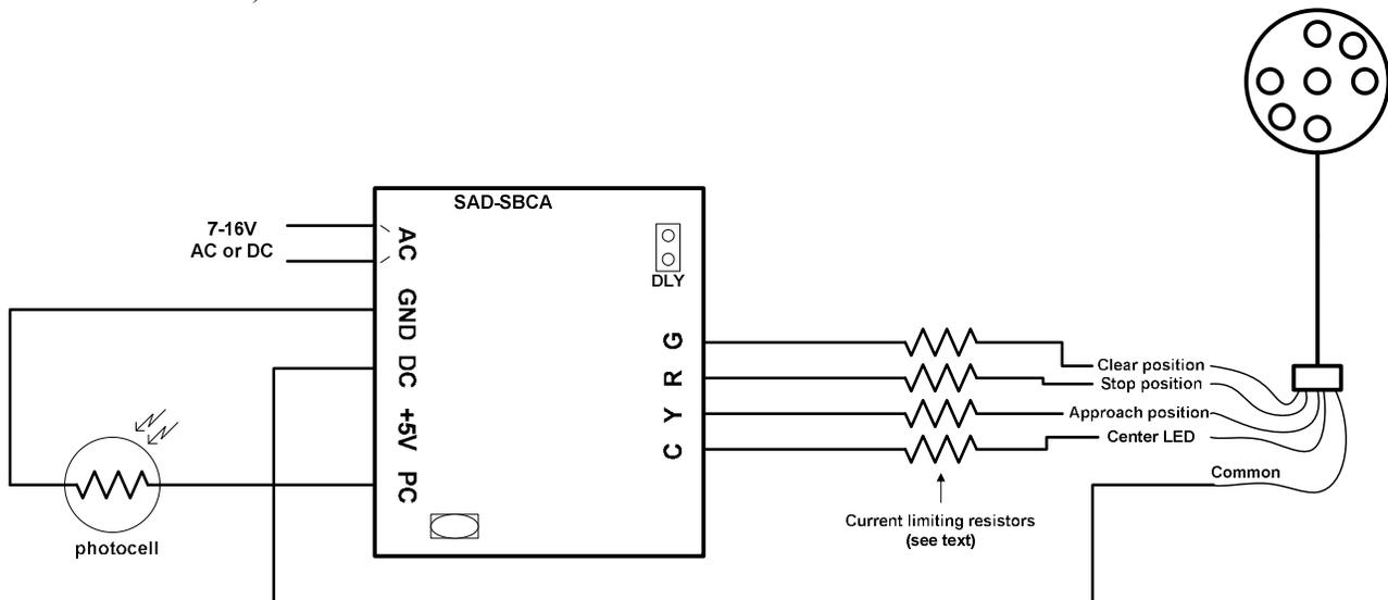
Figure 6 – LED-based position light signals (common anode wiring)
