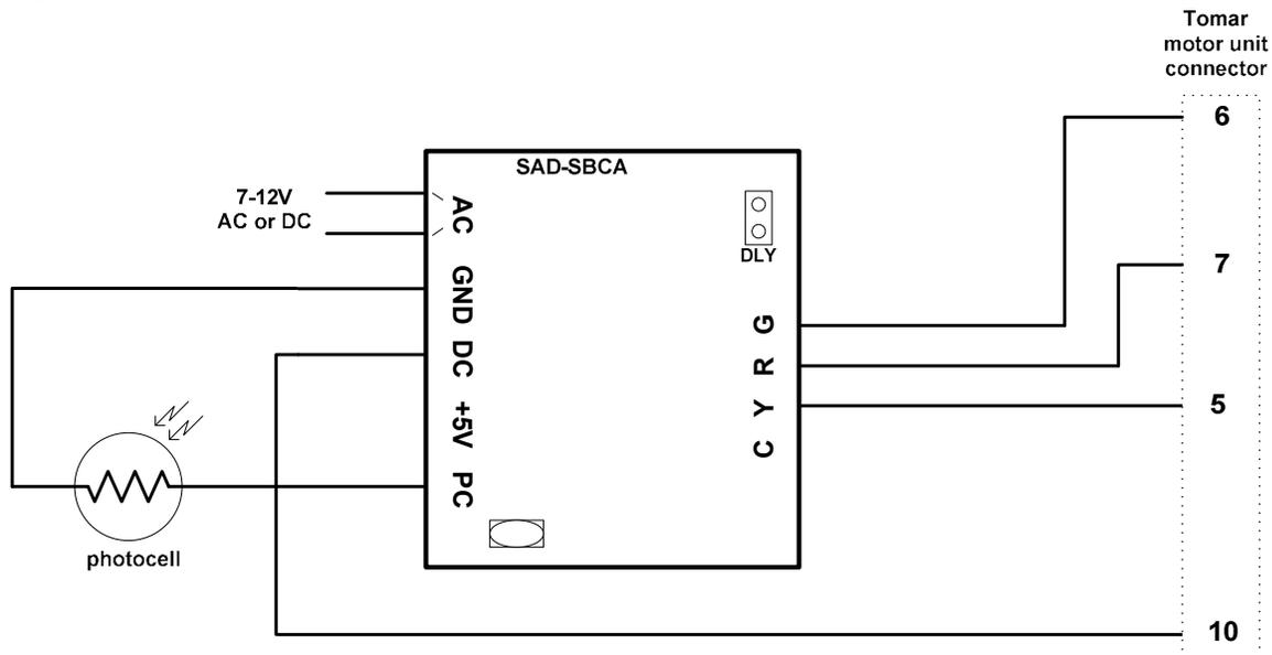
Figure 1 – Tomar semaphore motor connections
