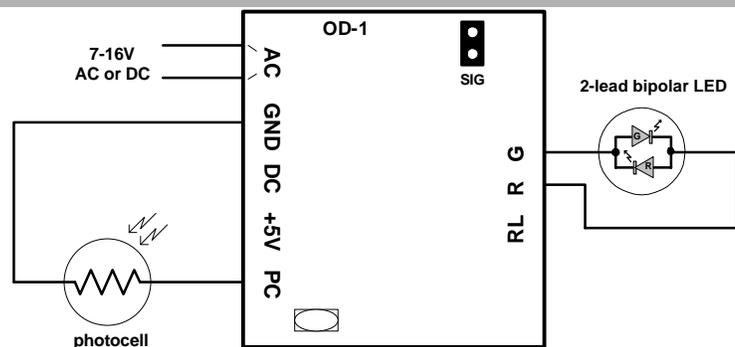
Figure 1 – 2-lead bipolar LED
