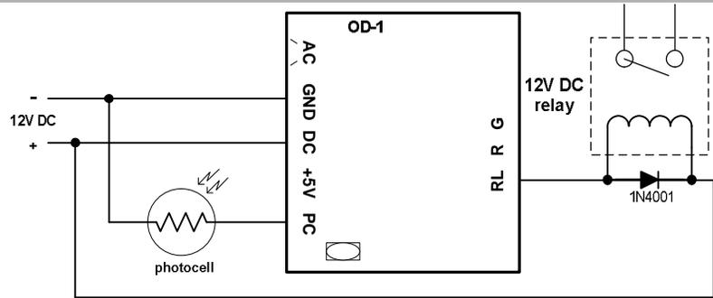
Figure 4 – Driving a relay
