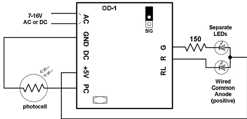
Figure 3 – Individual Red and Green LEDs (common anode)
