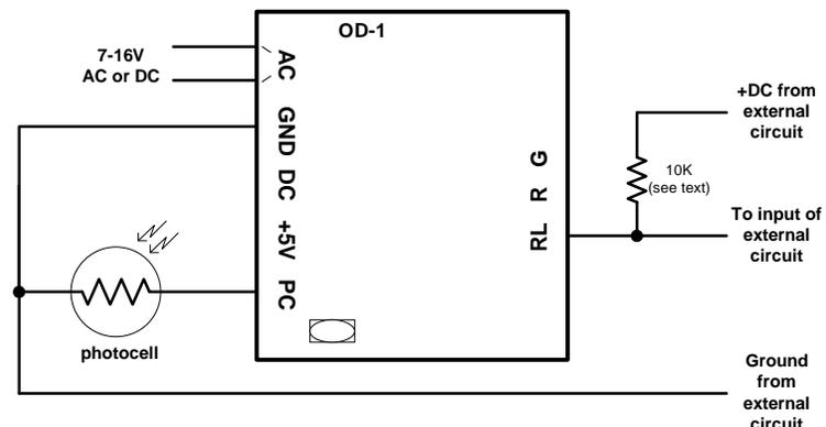
Figure 6 – Interfacing to an external circuit
