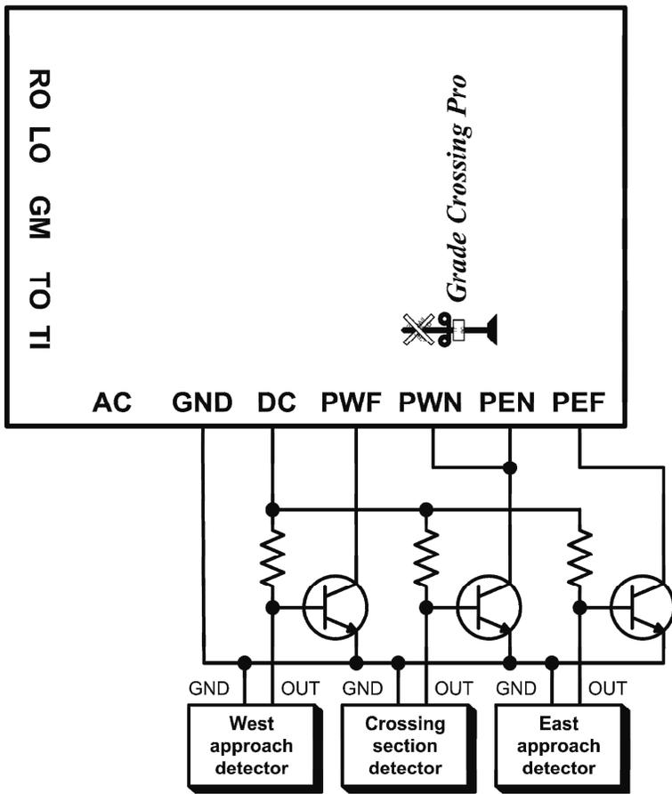
Figure 1 – Wiring for a GCP that came with photocells
