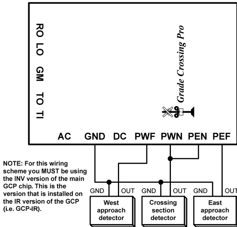
Figure 2 – Wiring for a GCP that came with infrared components
