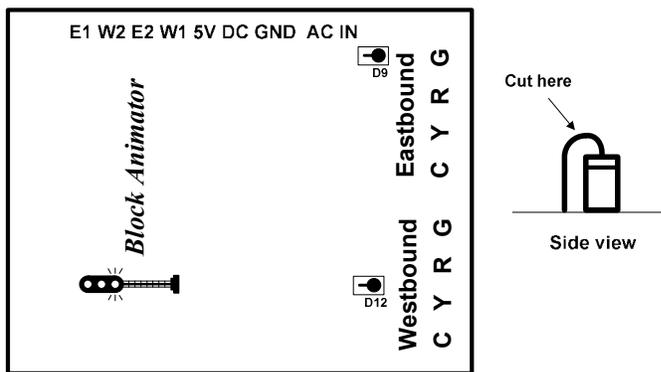
Figure 5 – cutting diodes for absolute type signals
