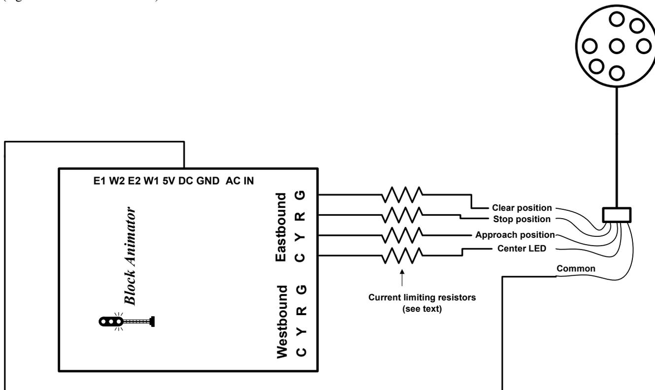
Figure 6 – LED-based (common anode wiring) position light signals
