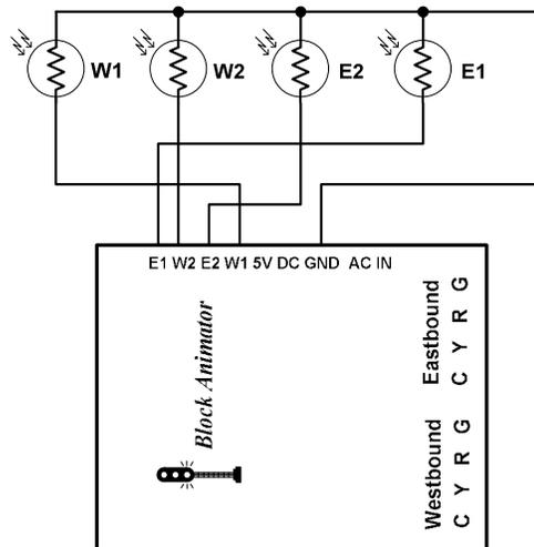
Figure 8 – photocell wiring
