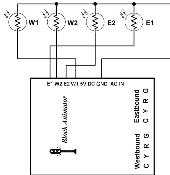
**Figure 5 – photocell wiring**
