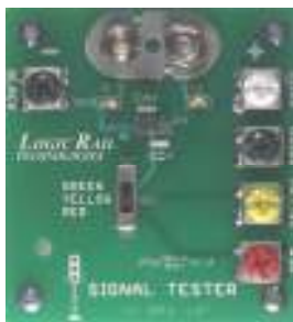
Figure 1a – ST-1 before battery installation
